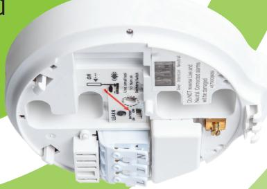
The FireHawk FH550RF Radio Base is designed to replace the baseplate supplied with the 250 and 450 ranges of mains powered smoke and heat alarms. When assembled to a maximum of 15 smoke or heat alarm on any one system, it allows the installer to power them all from a regularly used local lighting circuit (BS 5839-6:2013 section 15.5) without the need to run a separate interlinking wire.
